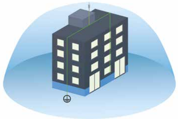
Illustration of area protected by Forend ESE lightning rod.
