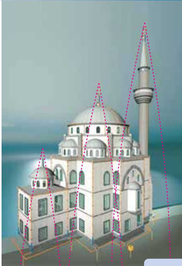
Protection zone provided by a Faraday Cage
